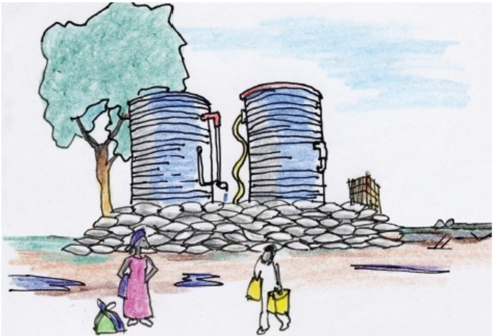
Elevated water reservoirs using sand bags
