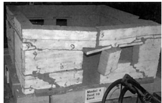
4-1 to 4-3 Typical failures caused by seismic movements (Tolles et al. 2000)
