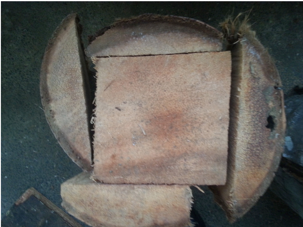
OLD CUTTING PATTERN TO GET "TABLONE" OUT OF CENTER, LOOSING MOST OF THE "A" GRADE MATERIALS IN THE CUTS THAT ARE THROWN AWAY
