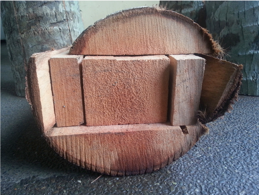
NEW CUTTING PATTERN PRODUCING A SMALLER TABLONE CONSISTING OF THE C/B GRADE MATERIALS, OUTER CUTS REMOVING SOME BARK, AND FOUR PIECES OF MIXED A/D GRADE MATERIALS FOR FURTHER REFINING AT SAWMILLS.
