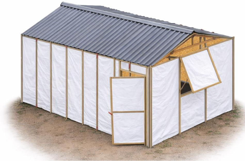
With internal cladding only
