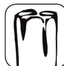
The water enters inside the culm causing fungal attack.
