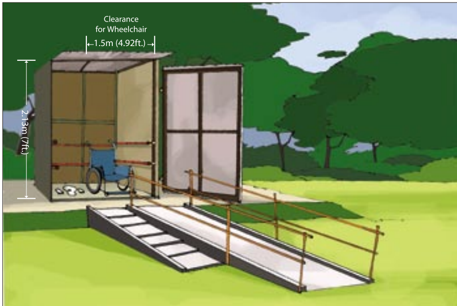
Accessible toilet with ramp, large door, and handrail along with space inside to accommodate wheelchair. Ramps can also be made adding a small slope to the level of latrine's floor.
