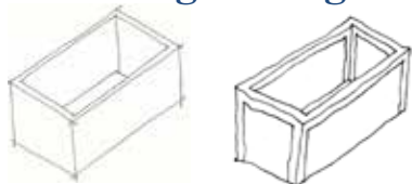
Walls with no RC column or structure with long spans are weak, walls should be plastered to enhance stiffness
