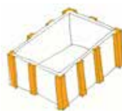
Adding pilasters to the walls
