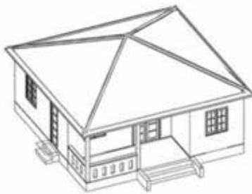
Use roof with four slopes (hipped roof)
