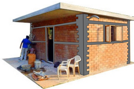
Confined Masonry House with clay brick walls and RC slab
