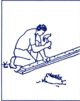
Make bearers using two 6 x 2's
