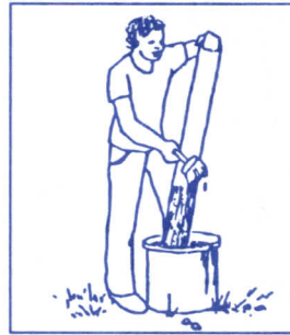
Paint them with wood preservative
