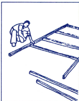
Nail studs to top and bottom plates on the ground
