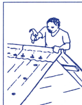
Put nail in each ridge of tin sheet
