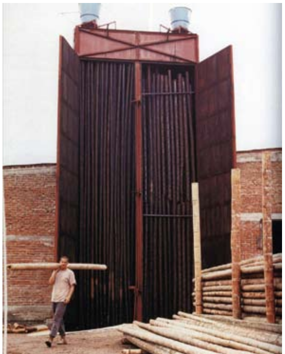
Oven used for smoke-imregnating bamboo poles 12
