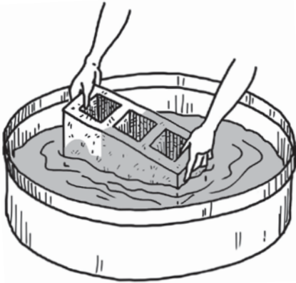
Soak the blocks in water for a while...
