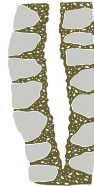
STONE WALL DELAMINATION WITH BUCKLED WALLS
