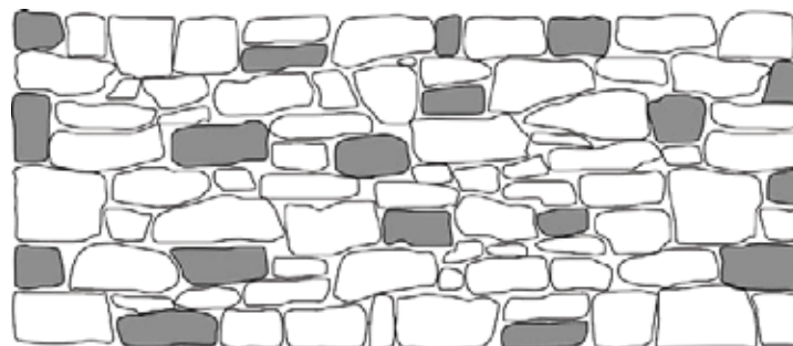
Good distribution of the through stones in the wall.
