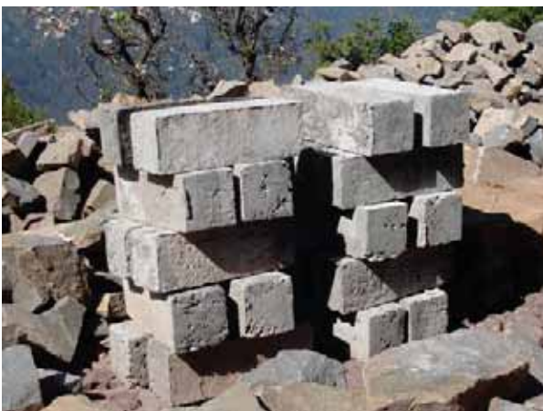
The corner stones can be replaced by reinforced concrete blocks made on the site.
