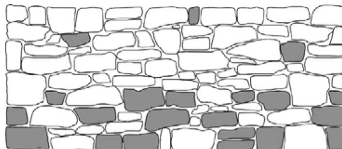
Bad distribution of the stones in the wall: all the through stones have been used at the beginning, resulting in a weak top of the wall
