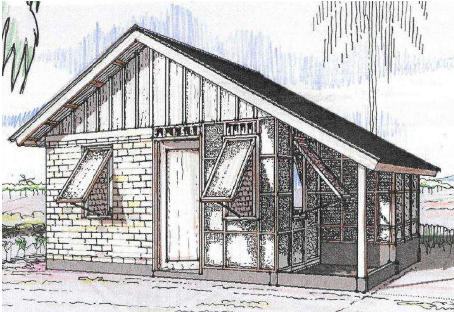
Hybrid house made of ICEB core and a timber component
