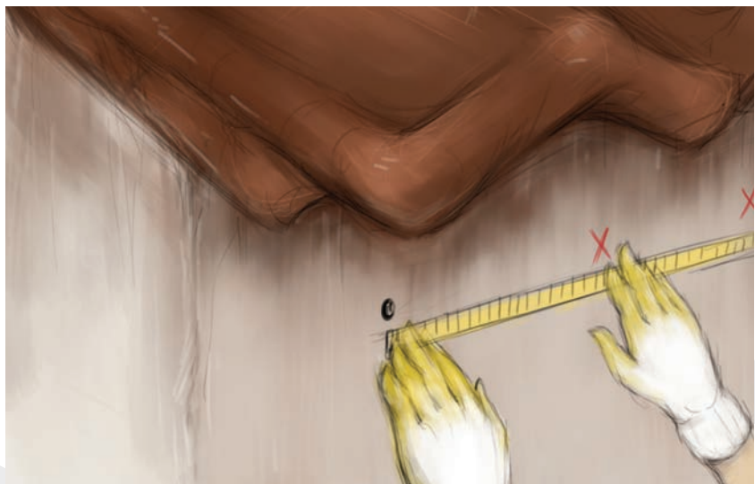
▶ Measure the distance between the holes in the plastic sheeting and mark the location of the nails on the wall accordingly.
