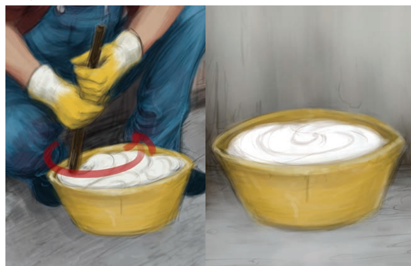
▶ Mix the water and gypsum well until the mixture is semi-liquid and there are no lumps. The mix should be used as soon as possible, otherwise it will begin to harden.
