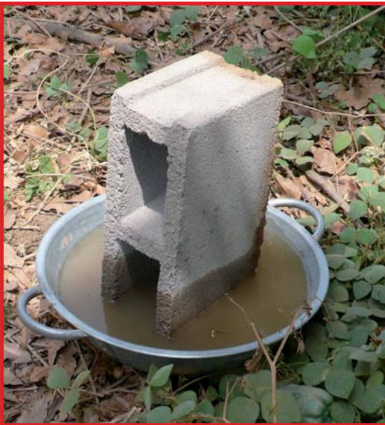
Water rising up due to capillary
