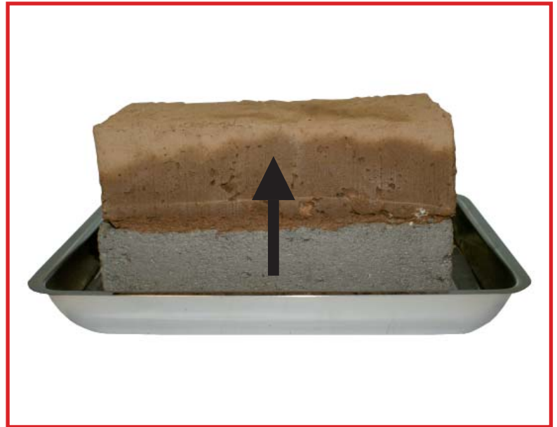
In spite of a water-resistant basement, water rises up to the earth walls
