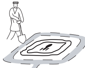
curtain drain - trench dug around the latrine
