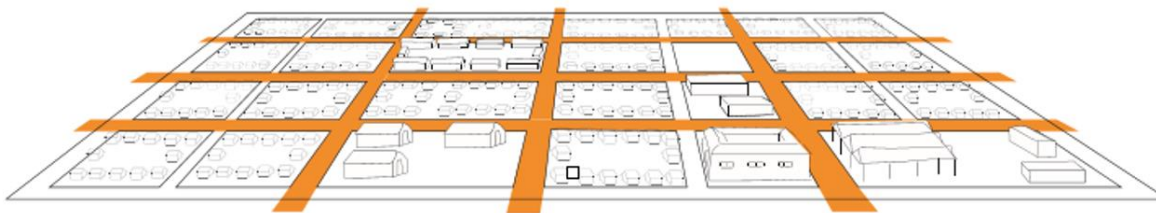
Image 1: Access for emergency vehicles can be achieved through simple grid system
