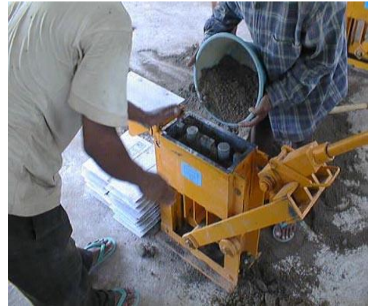
HI - CSEB Block machine - Habitech centre, Thailand
