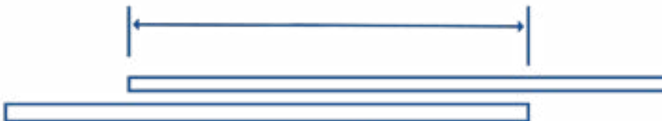
TYPICAL MINIMUM LAP SPLICE FOR REINFORCING BARS
