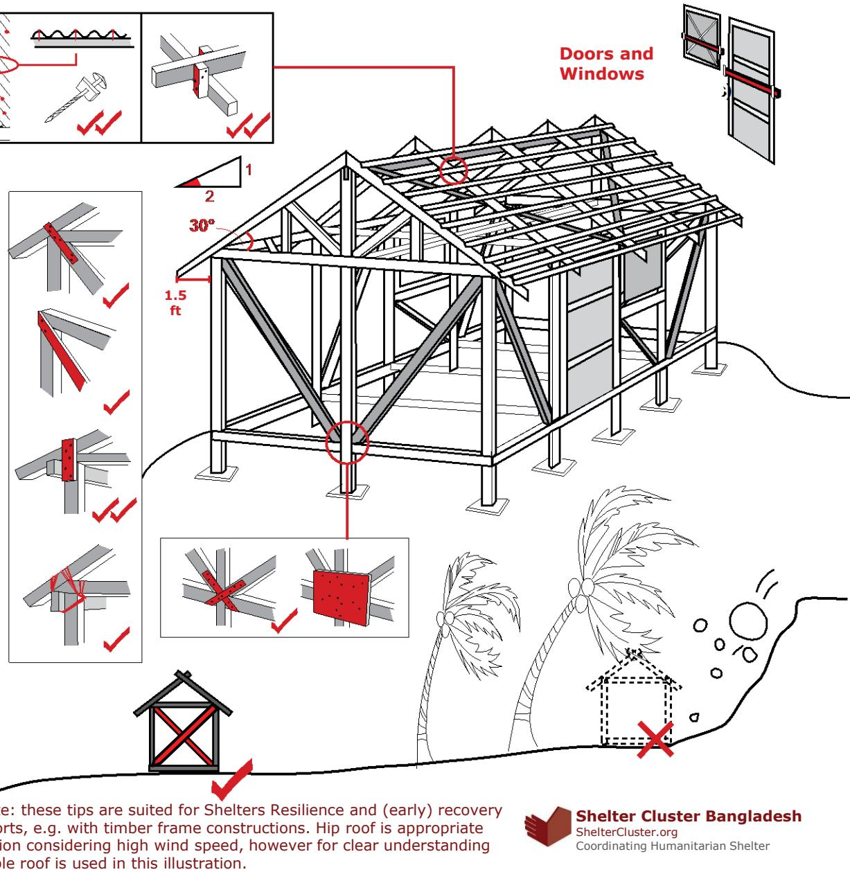
Note: these tips are suited for Shelters Resilience and (early) recovery efforts, e.g. with timber frame constructions. Hip roof is appropriate option considering high wind speed, however for clear understanding gable roof is used in this illustration.
