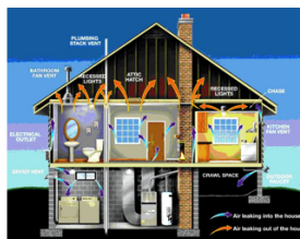
Figure 33 Classic air leak affecting insulation performance
