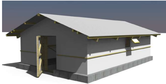
PHASE 2 Replacement of Bama Shelter roofing with CGI sheet, and Reinforcement with Sand Crete block work round
