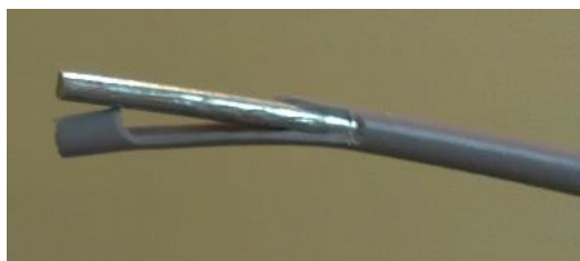
Left: A sample of thick PVC coated galvanised wire found in Tacloban. (Photo: R. Dodds)
