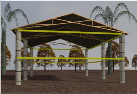
Scissor trusses, CRS design 2014
