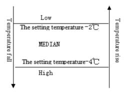
When the difference between the setting temperature and the room temperature equal to 2 or 4 , the indoor fan speed will keep in current speed.
