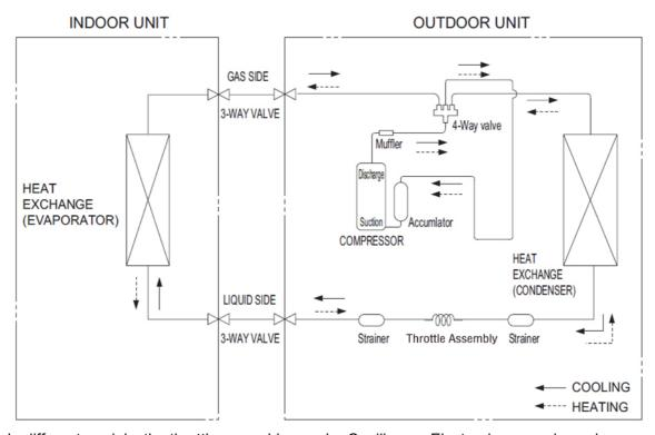
NOTE: In different models, the throttle assembly may be Capillary or Electronic expansion valve.
