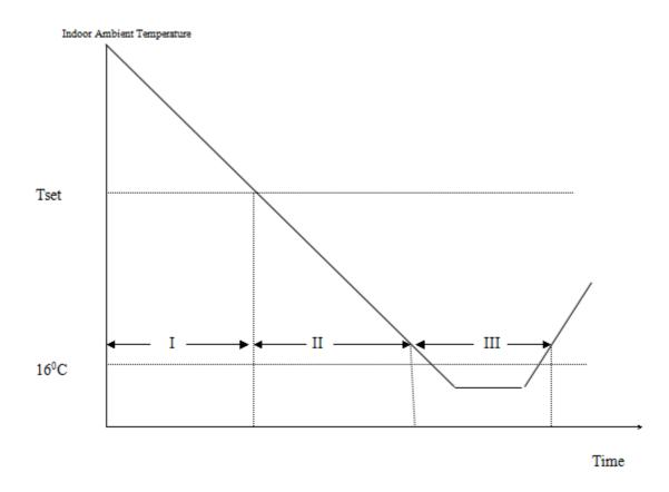
Dehumidifying area I: Operation at the frequency in the range (30–60Hz) according to Dt ( $T_{indoor}$  ambient- $T_{set}$ ).
