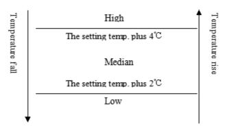
When the difference between the setting temperature and the room temperature equal to 2 or 4 , the indoor fan speed will keep in current speed.
