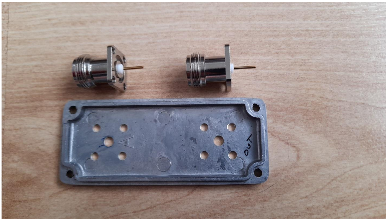
Figure 2 Lid drilled correctly for N-Type connectors
