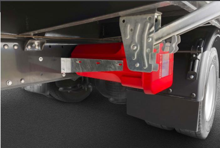
This fire extinguisher cabinet is designed for use with commercial vehicles and is manufactured from injection moulded polypropylene. The reinforced and non-deformable structure guarantees strength. These cabinets are designed for mounting horizontally or vertically on the vehicle. With the top loading design, they are the perfect solution when space is restricted.
