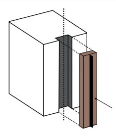
To achieve excellent adhesion seals must be applied to clean, dry surfaces at temperatures between +5°C and +40°C.
