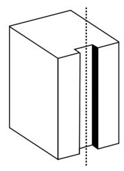
Measure and cut seal to length using a hacksaw. Remove self-adhesive backing and butt joint fit all seals to inside and outside of door frame or door, and meeting stiles of pairs of doors where applicable.
