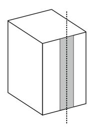
Rout a groove suitable for the size of intumescent seal selected. Clean the rebate to remove any dust.
