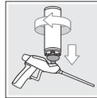
1. Shake the canister at least 20 times before each use and then screw onto the gun
