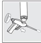
2. Adjust trigger and metering screw on the gun and apply AA005 Conical Adaptor (or similar) to end of foam gun
