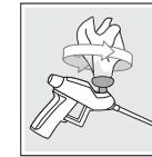
2. Clean the gun valve, nozzle and conical adaptor with a clean cloth
