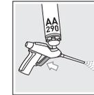
4. Press the trigger until the cleaner sprays through the nozzle
