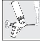
3. Set the discharge quantity by adjusting the dosing screw and apply the foam in a continuous application
