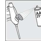
1. Remove all attachments from the gun and spray the gun valve, nozzle and conical adaptor with the gun cleaner
