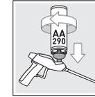
3. Screw the gun cleaner onto the gun
