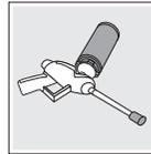
5. If leaving the canister for short breaks during use, close the nozzle on the gun and store the can vertically
