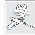
7. Repeatedly clean the gun valve, nozzle and conical adaptor with a clean cloth until thoroughly clean
