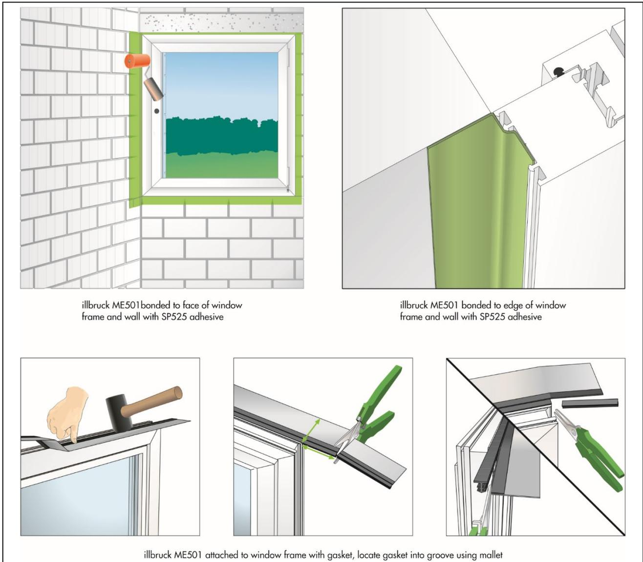
**Bonding with SP525 Adhesive after frame installation** (suitable for single windows and curtain walling/multiple coupled windows/assemblies) (see Figure 5).
