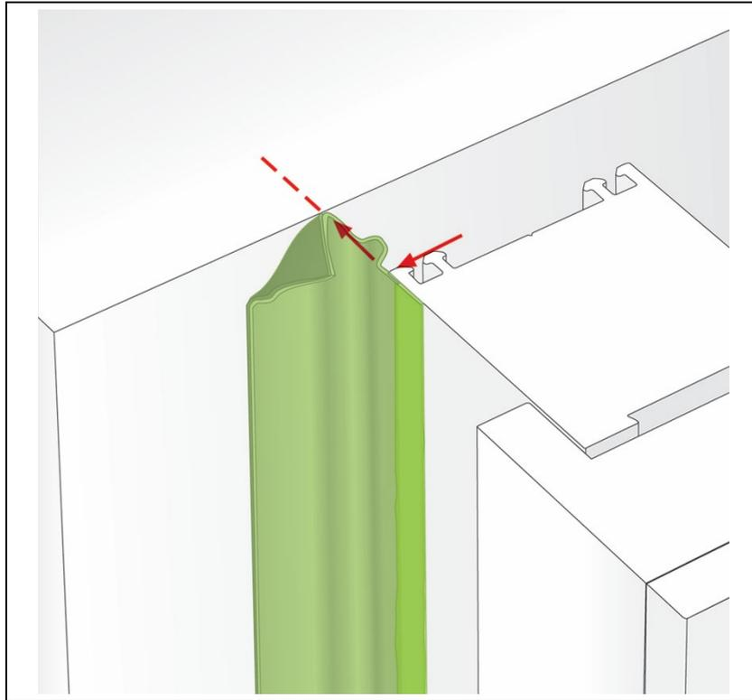
17.2 Application is continued around corners, carefully folding to ensure continuity of the membrane, ensuring that no radii are present at the corner interface with the internal blockwork or other construction material.
