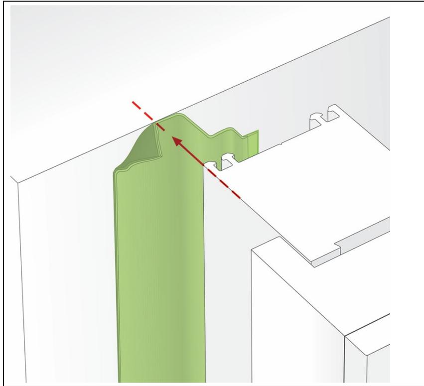
18.2 At each corner, the membrane is bent and folded to ensure that the acrylic self-adhesive strip is back-to-back, leaving an extra 20 mm length (40 mm of membrane) at all corners.
