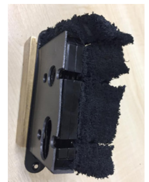
Expanded Pyrolock graphite intumescent before and after.
