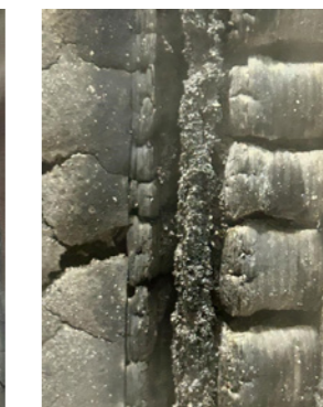
Expanded graphite in the gap between doorleaf and frame.
