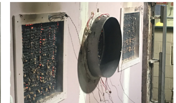
Thermocouples monitor the temperature on the non fire side to establish if the insulation criteria is achieved.
