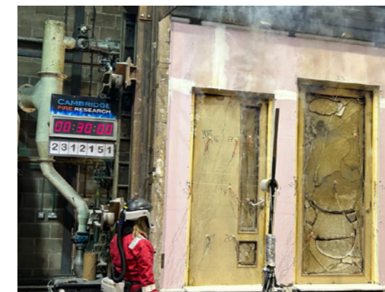
A successful test for 30 minutes has been achieved here for these 30 minute doors fitted with KuhnOdice's Pyrostrip, Pyrohinge, Pyrolock, Pyrocloser and Pyroglaze products.
