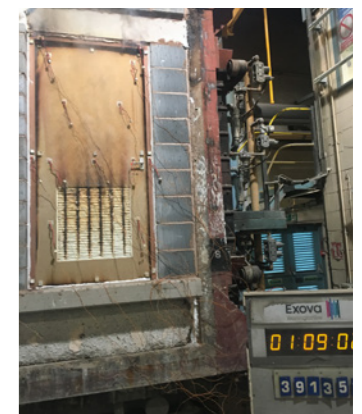
This FD60 test with a large Pyrogrille ATG has already clocked up over an hour and is still going strong.
