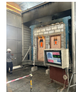
These fire doors achieved 98 minutes on a 90 minute fire test.
