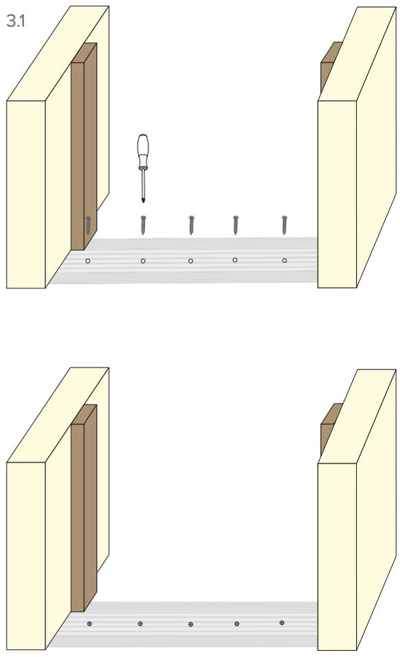
**3.1** Place threshold in position and using the screws and plugs provided screw the threshold into place ensuring the screws are flush with the threshold.
