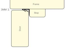
**2.1** Place adhesive edge on the frame with the rear blade against the door stop. Fit the NOR710 from the top to the bottom of both sides then fit to the top ensuring the rear blade is against the door stop. Trim to size with a sharp knife. Ensure the gap between the door and frame is 3mm
