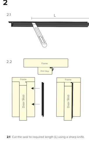
2.2 Peel off self adhesive backing and gradually push fit the seal into the groove up both jambs and head of the frame. (Note, The seal must not impede the opening and closing of the door)
