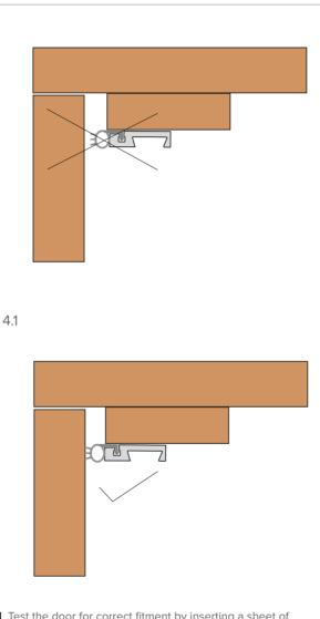
**4.1** Test the door for correct fitment by inserting a sheet of paper between the door and the door seal. Shut the door and adjust the seal to ensure a consistent seal all around the door. Note the door should firmly hold the sheet of paper
