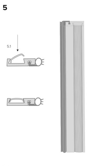
**5.1** Once installed correctly, fit the cover cap over the screws by inserting one end first then the other.
