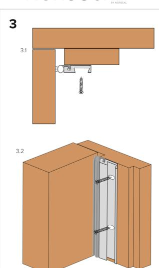
3.1 With the door closed. Position the seal at the head of the door first, The seal should just rest against the door lightly. Screw into the centre of the elongated holes of the holder so adjustment can be made if needed.
