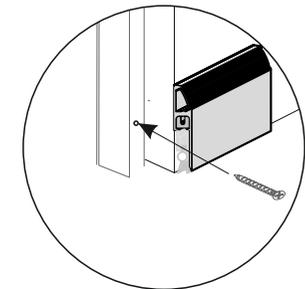
**2** With the door open, Screw the drop seal to the door and then screw the actuator into position. Then replace the screw cover.
