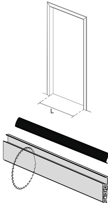
**1.1** Measure the inside of the door (L) Remove the screw cover, then cut the seal to size to a max of 150mm from either side. (NOTE, if only cutting one side you must cut the NON actuator side)
