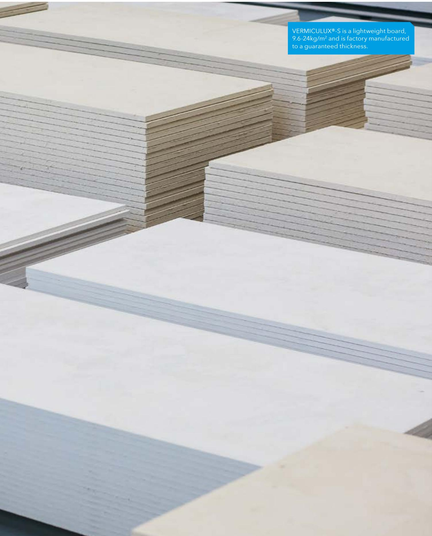
VERMICULUX®-S is a lightweight board, 9.6-24kg/m<sup>2</sup> and is factory manufactured to a guaranteed thickness.
