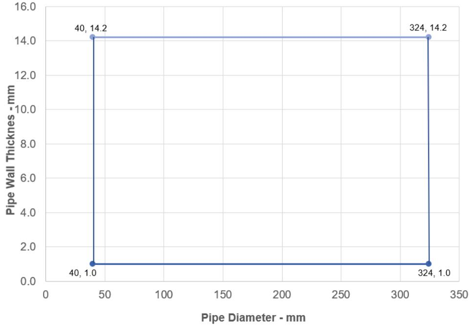
**Copper or Steel Pipes with 30-80 mm Thick Insulation
