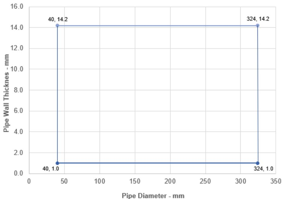
**ALUPEX Pipes with 30 mm Thick Insulation - EI 90 C/C**
