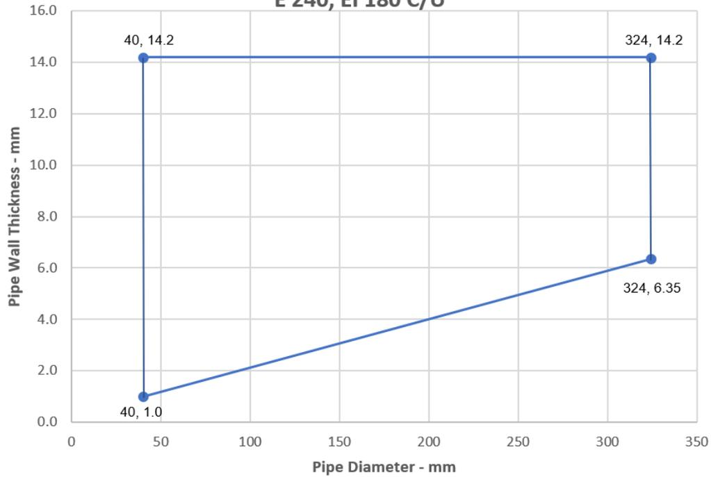
**ALUPEX Pipes with 30 mm Thick Insulation - EI 240 C/C**
