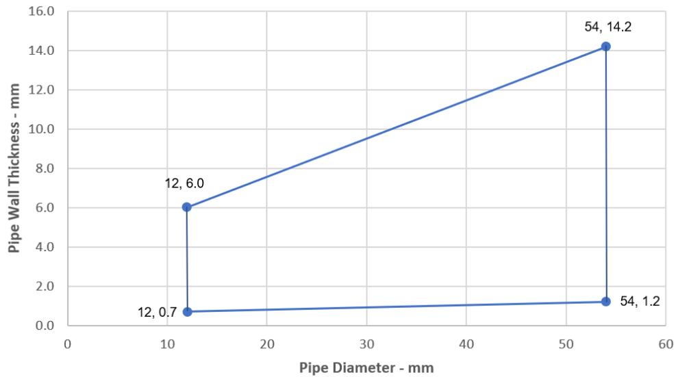
**Alupex Pipes with 30-80 mm Thick Insulation
