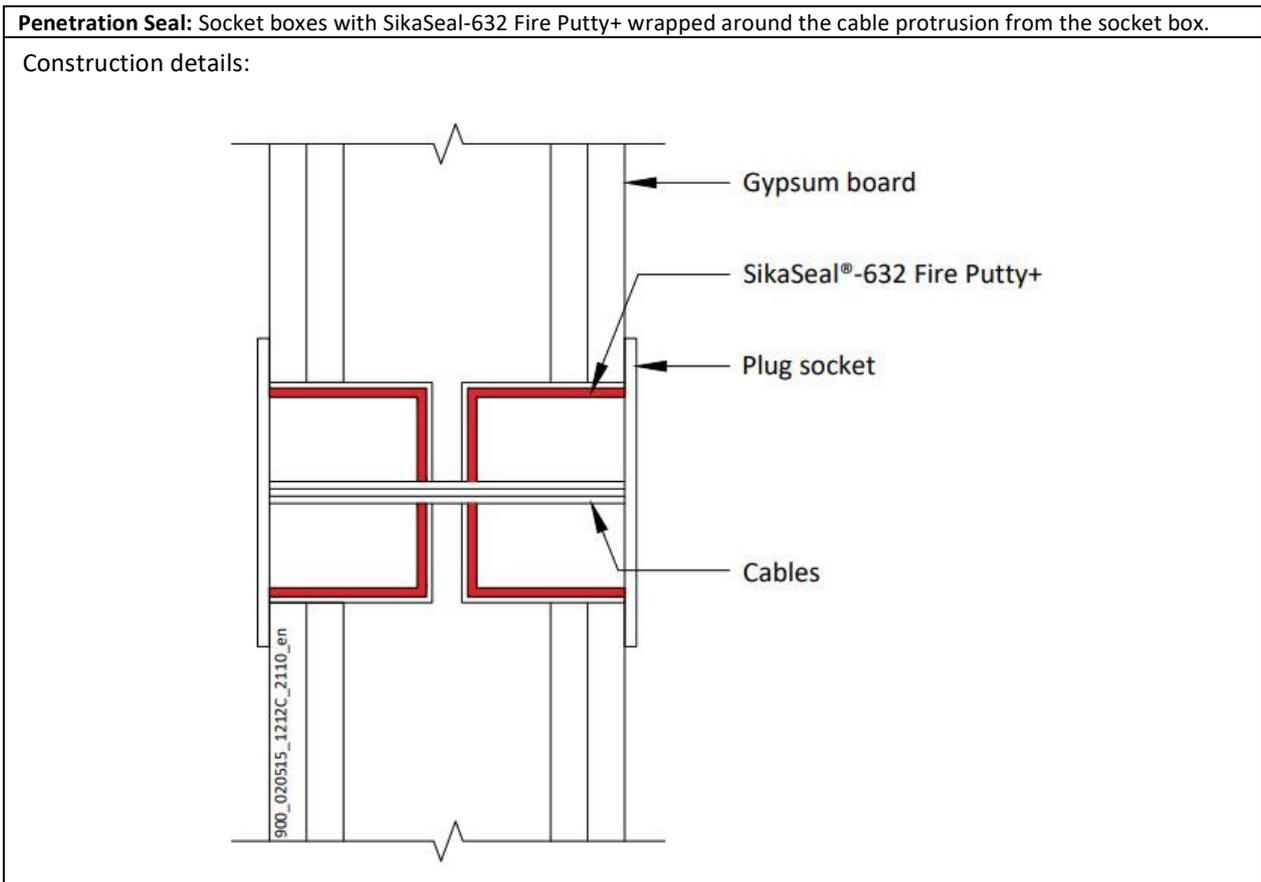
**A.2.1.1 Double side penetration seal with cables in socket boxes**
