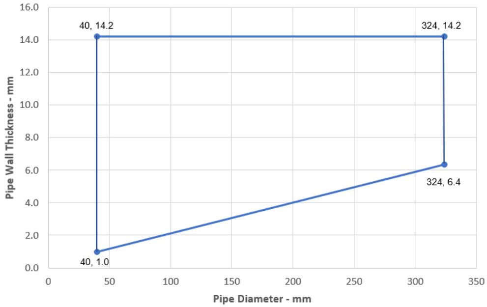
**Copper or Steel Pipes with 30-80 mm Thick Insulation
