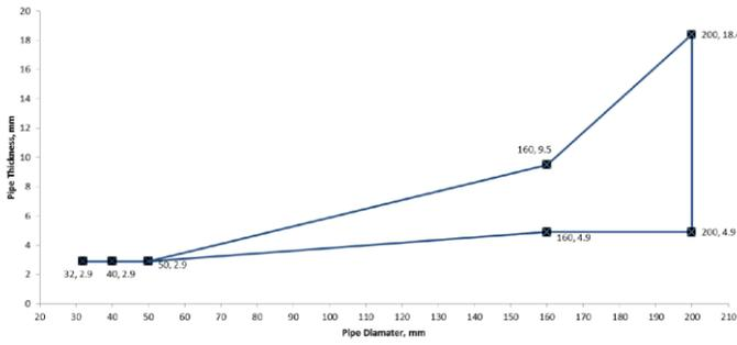
Plastic Pipes PE according to EN ISO 15494, U/C, wall ≥ 100 mm - EI 90
