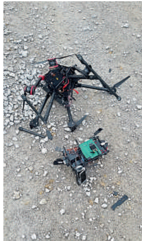
Crashes do happen! This is the result of a motor failure at a recent mine site mapping project
