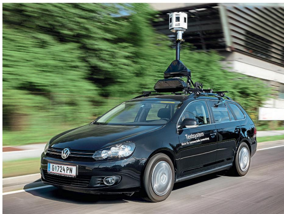
The UltraCam Mustang vehicle-based mobile mapping system represents a proven, state-of-the-art system for capturing street-level georeferenced panoramic imagery and 3D data
