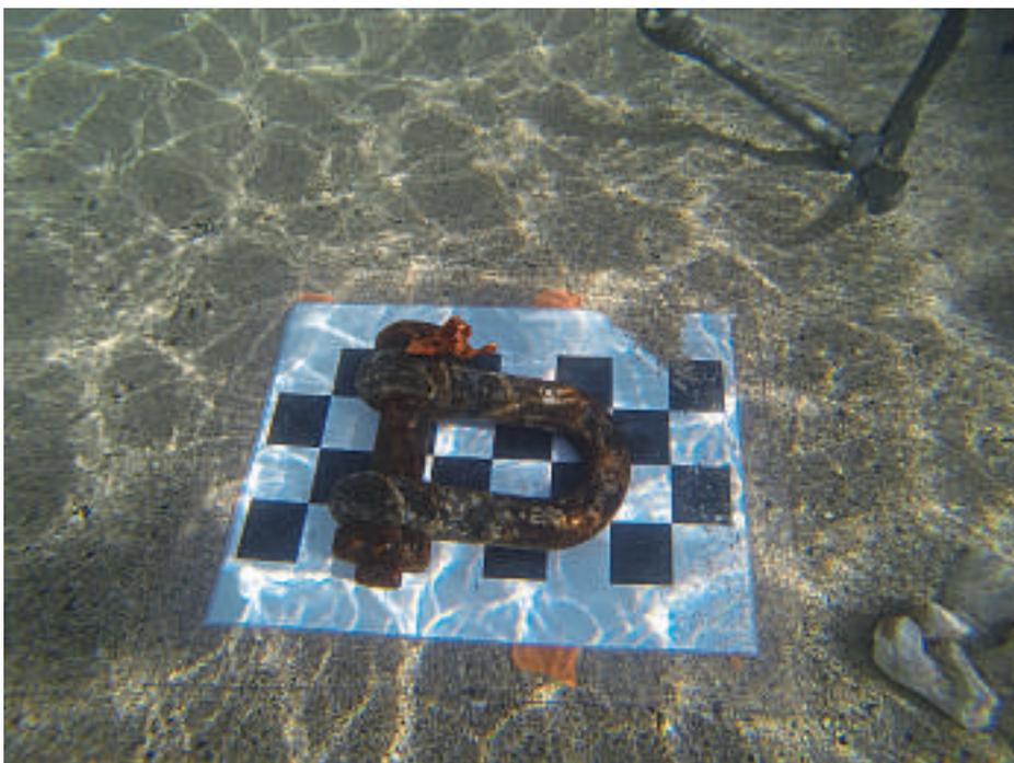
Figure 5. Light patterns change due to the water surface waves
