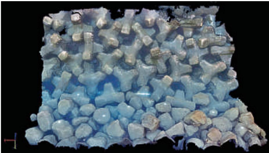
Figure 4. Metal scale bar and tags placed in the mapped area to be used in Pix4Dmapper Pro as a scaling tool and as GCPs
