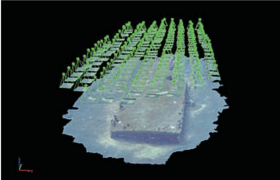
Figure 3. An image acquisition plan that ensures consistent image overlap
