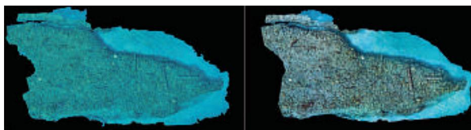
Figure 8. Comparison of a 3D model generated with a set of original images (left) and with colour-corrected ones (right)
