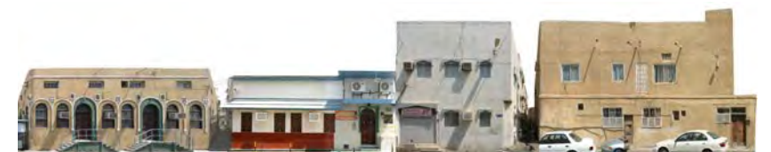
Typical street elevation using rectified photogrammetry.
