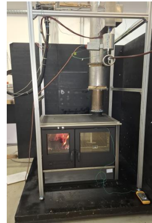
Picture of fuel batch in combustion chamber
