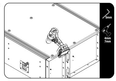
Remove the Fridge Slide and Drill a 7mm hole through the wood on each of your markings. Loosen and remove the deck.
