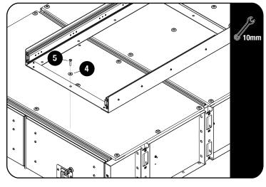
Secure the Deck back onto the drawer system. Place the fridge Slide (Item 1) back into position and secure using M6 x 20 Hex Bolts and M6 x 19 x 1 Flat Washers (Items 4 & 5).
