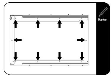
Place the Fridge Slide (Item 1) on the suitable surface, open the slide and mark the positions as shown as indicated by the arrows (at least 6 fixing points recommended).
