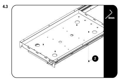
The M6 x 16 Button Head Bolts (Item 2), supplied are used to secure a Dometic Fridge.
