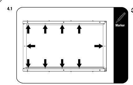
Place the Fridge Slide (Item 1) on the suitable surface, open the slide and mark the positions as shown as indicated by the arrows (at least 6 fixing points recommended).
