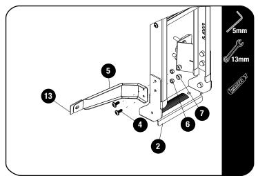
Assemble the Spare Wheel Mounting Bracket (Item 5), by sticking the Foam Rubber (Item 13) on the back of the bracket as shown and trim it down to the shape of the bracket.
