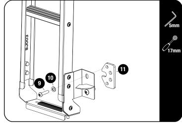
Secure the Ladder Hinge Mount Bracket to the hinge using M8 x 35 Button Head Bolts, M8 x 16 x 1.6 Flat Washers and the Hinge Spacer (Items 9, 10 & 11)
