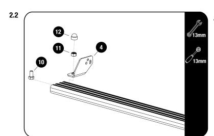
Fit the Light Bar Bracket 01 LH / RH (Item 4) for for the 40" Light Bar, using M8 x 16 Hex Bolt & M8 Nyloc Nut (Items 10 & 11). Fit the light bar and center it on the slat before fully tightening the brackets.
