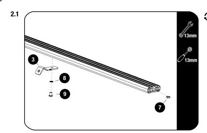
Slide one M8 Thin Nut (Item 7) into the T-Slot of the front slat. Center the Mid Support Bracket (Item 3) in the Middle of the slat and secure using a Schnorr Washer and M8 x 12 Button Head Bolt (Item 8 & 9). Fully tighten.
